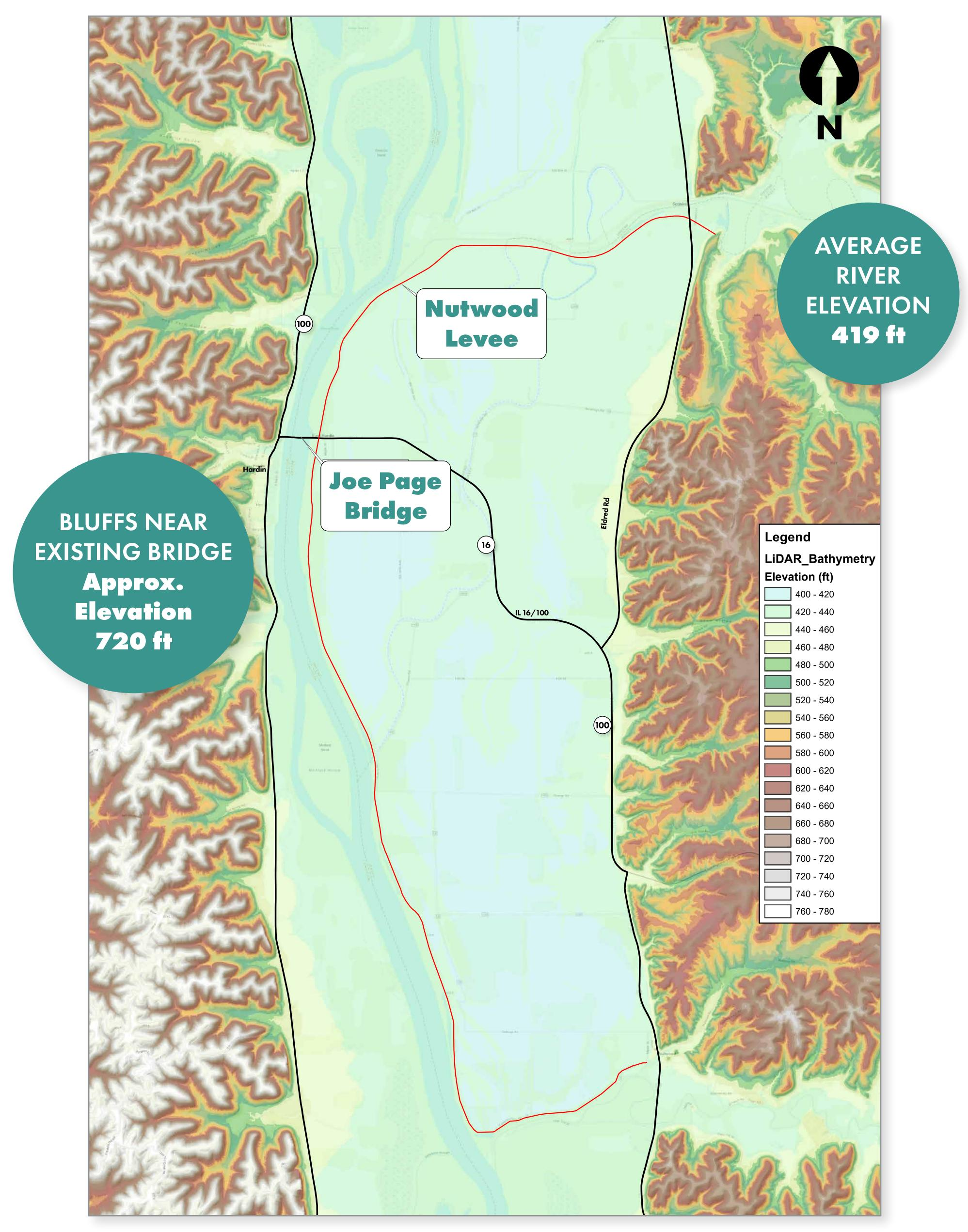
This elevation map helps show the height difference between the top of the bluff and the IL River. Normal Pool for the IL River is at elevation 419, indicated by the blue color on the map. Some bluff locations near the existing Joe Page Bridge have an approximate elevation of 720, indicated by the grayish brown color on the map. This component must be considered as a location for the new bridge is evaluated.
